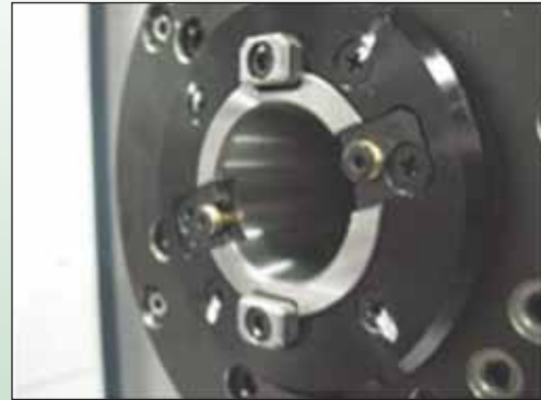
Taper face tool's axial position is maintained even at high rotational speed.
