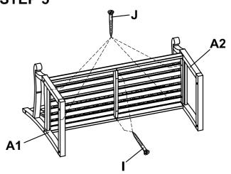
Secure the seat (C) using 1 1/2" screws (I) and 1" screws (J), as shown.
