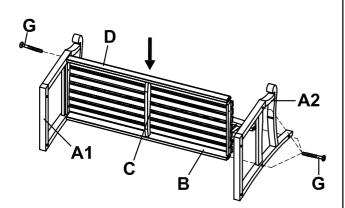
Attach the front apron (D) into seat (C) and right side frame (A1) and secure using 1 1/2" bolts (G). Next, attach the left side frame (A2) into back support (B) and front apron (D). Secure using 1 1/2" bolts (G).
