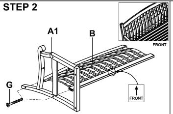
Attach the right side frame (A1) into back support (B). Secure with 1 1/2" bolts (G).
