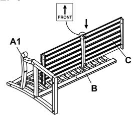
Next, attach the seat (C) into predrilled holes of back support (B).
