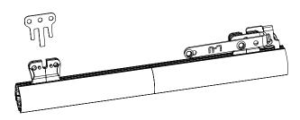
Step 5. Tighten the Splice set screws.
