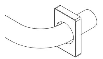
2. Use a 3/16" Allen Wrench to attach the Bracket Base onto the pole. The Bracket Base can be aligned vertically or horizontally.
