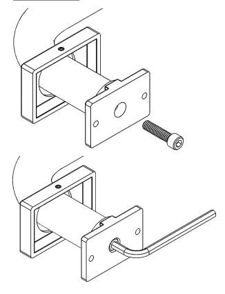
3. Attach the Bent Return Pole Assembly to the wall. Use hollow wall anchors if not screwing directly into a wall stud. (Vertical Installation Shown)
