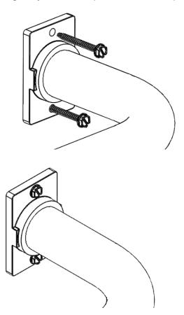
4. Slide Bracket Cover onto Bracket Base and tighten the set screw with the Allen Wrench provided to hold the cover in place. Repeat for the other bracket. (Vertical Installation Shown)
