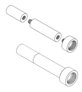
3. Place the base cover over the base and hold in place while screwing the stem assembly onto the base. Tighten to hand tight only. (Shown without the stem extension option).
