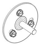
2. Screw the Tieback Finial Adapter onto the holdback stem.
