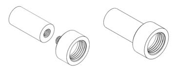
OPTIONAL: To add 2 inches of length to the Tieback stem. Screw the Tieback Stem Extension into the Tieback stem, and then screw the finial adapter into the stem extension.
