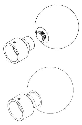
2. Slide the Finial & Collar Assembly onto the Pole and tighten the set screw with the Allen Wrench provided to lock into place.
