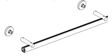
Step 5. Tighten all wall mount stems with set screw located above the wall mount cover.
