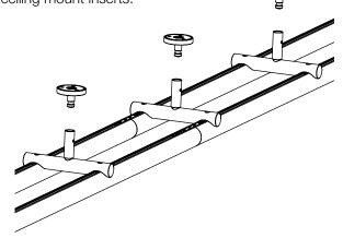
Step 6. Tighten all ceiling mount stems with set screw located close to the ceiling mount cover.
