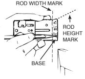
Step 3 Center punch (a small nail will work) and drill holes at all marks. Hole size depends on which fasteners you choose from the "FASTENER GUIDE".
