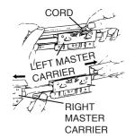
Step 4 If your draperies will OPEN TO THE RIGHT, remove the slides from the left of the master carrier by pressing down on the spring gate and sliding them out of the rod.
