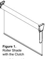
mount the brackets as close to window as possible yet have enough space for the shade fabric when completely rolled up. The shade can be regular wind or reverse wind as shown below
