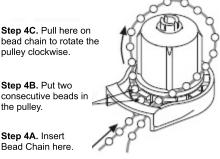
Step 4A. Insert Bead Chain here
