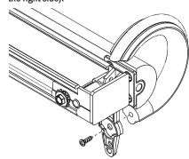
13. Lift the track assembly onto the wall brackets and secure in place.
