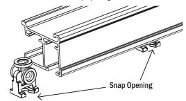
Install the end caps onto the track. (Left side shown - repeat for the right side).
