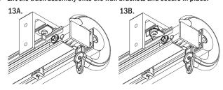
14. Snap the "C" Rings onto the roller carrier bodies.
