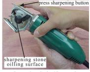
Figure 2. Blade Sharpening
