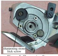
Figure 5. Sharpening Stone
