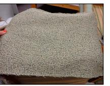
Trim and push fabric into the teeth of the tack strip and staple the bottom to the frame.
