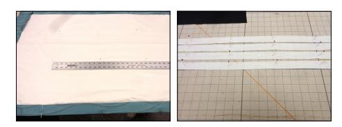
At the table, tuck a length of lift material into the bottom hem for each row of lift. Pin.
