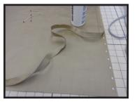
At the machine, sew the welt to the face piece, making the join in the covered cord as you come to it.
