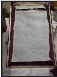
**14** Lay in a layer of batting, making sure no batting gets in the tack strip teeth. Staple sparingly.
