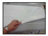
At the machine, sewing on the face, sew on one side of one row of welt, from top to bottom.
