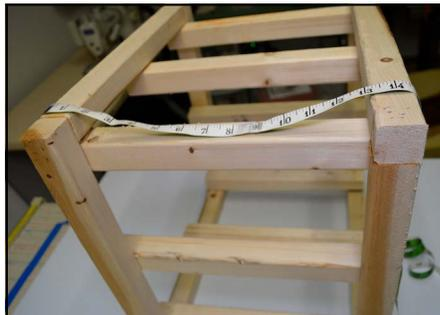
2 Cut two pieces of FirmaFlex™ to the width and height measured. This will be a rectangle.
