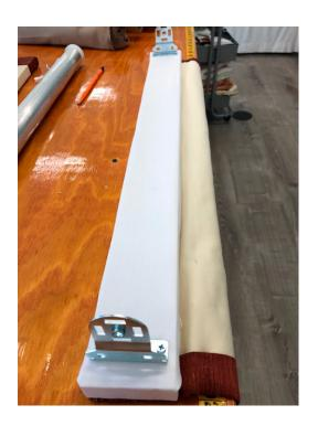
Complete the shade in your method of choice. Insert the prepared shade tube into the brackets. Add the cord clips to the shade tube.
