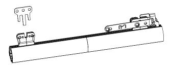
Step 5. Tighten the Splice set screws.
