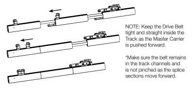
Step 4. Bring both Master Carrier Body halves together and insert the center clip.
