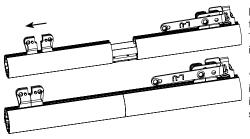
NOTE: Keep the Drive Belt tight and straight inside the Track as the Master Carrier is pushed forward.
