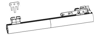
Step 5. Tighten the Splice set screws.
