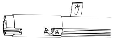
NOTE: Glides can be added or removed with the Drive Pulley installed by removing the End Stop.
