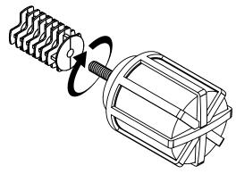
2. Insert the plug into the pole and push firmly until the plug fits entirely into the pole (do not use a hammer or any other method to pound on the finial).
