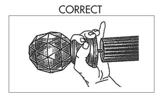
DO NOT hold finial by the crystal when installing into pole.
