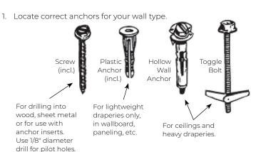
IMPORTANT: We suggest always installing brackets into wall studs for added security. If not installing into wall studs, be sure to use appropriate fasteners for your wall type.
