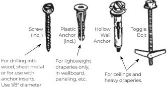
IMPORTANT: We suggest always installing brackets into wall studs for added security. If not installing into wall studs, be sure to use appropriate fasteners for your wall type.
