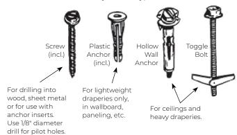
IMPORTANT: We suggest always installing brackets into wall studs for added security. If not installing into wall studs, be sure to use appropriate fasteners for your wall type.
