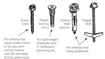
IMPORTANT: We suggest always installing brackets into wall studs for added security. If not installing into wall studs, be sure to use appropriate fasteners for your wall type.
