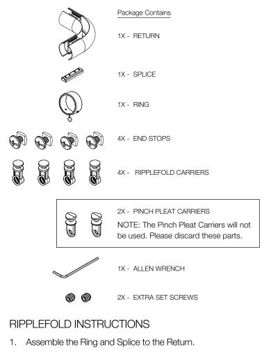
NOTE: To change the handing of the part simply assembly components on the opposite side.
