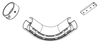
2. Assemble the Ripplefold Carriers and End Stops on to the Return.
