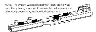
Step 2. Remove all packaging material from the Track, ensuring the Drive Belt stays in place inside the Track.
