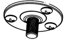
Step 3. Locate ceiling bracket cover. Place cover over the ceiling plate.
