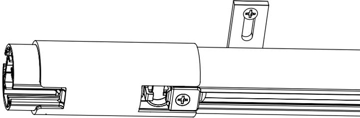
NOTE: Carriers can be added or removed with the Drive Pulley installed by removing the End Stop.
