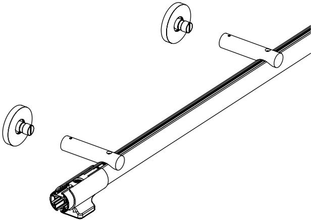
Step 5. Tighten all wall mount stems with set screw located above the wall mount cover.
