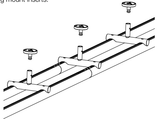
Step 6. Tighten all ceiling mount stems with set screw located close to the ceiling mount cover.
