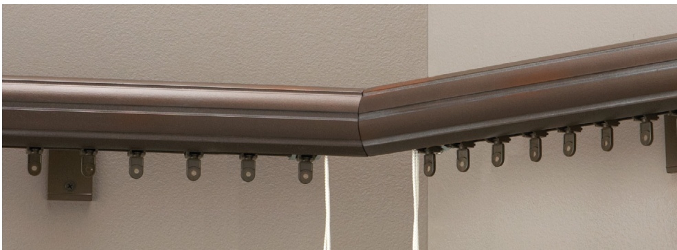
Shown: 120° mitered bay corner for corded traverse system, 225FL wood fascia, finish 740 Smoky Mocha; bronze track, bracket, and components
