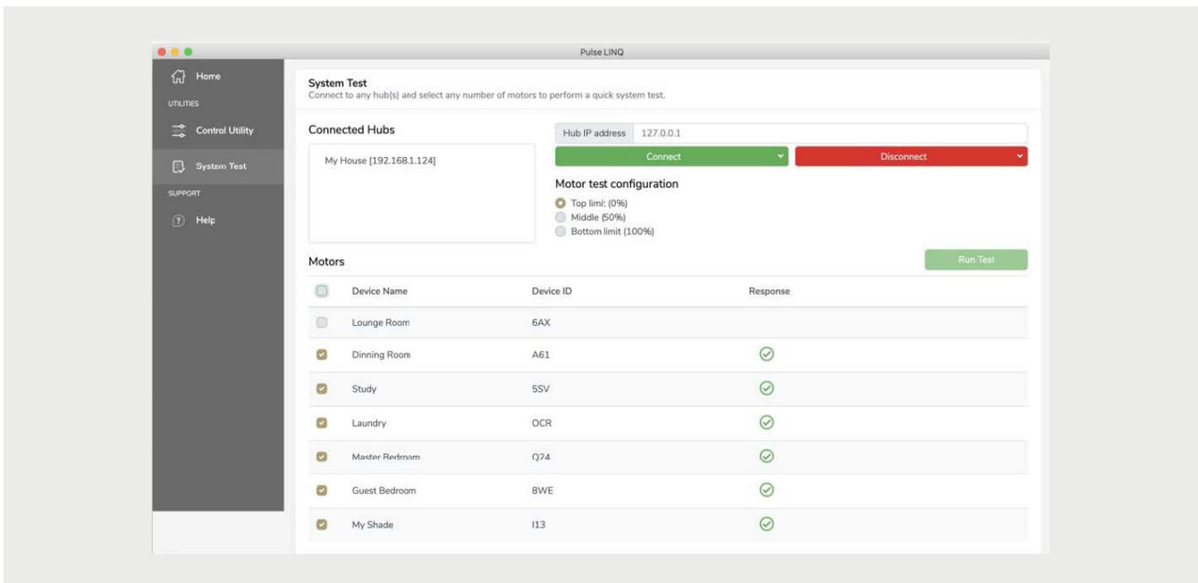
To run a system test you need to select the motors you wish to perform the test on then select the Motor test configuration option then Run Test.
