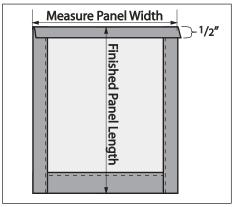
2. Measure the panel width. Cut a strip of cartridge pleat tape 2 times the panel width, plus 8" extra.
