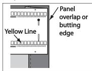
5. At the outer edge of the panel (opposite from the overlap or butting edge), trim the tape to 1" beyond the edge of the panel. Tie loose draw cords together for later pleating. If cords are not exposed, find a set of repeat indicating dots closest to the edge, use an opened paper clip to pluck the draw cords out and tie. Turn the tape 1" under.
