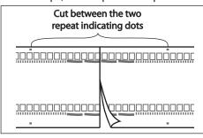
3. Remember, the two just cut tape ends will be located at where the two edges of drapery panels meet (at the center of the drapery rod). On both tape strips, next to the just cut end, free each exposed draw cords to where the cords disappearing into the tape, double knot, trim the tape 1" away from the knots.
