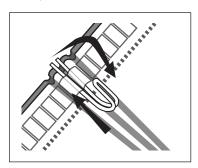
Insert the two-prong curtain hooks at both leading edges of the panel for overlap and return.
