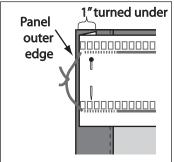
6. Machine stitch the tape to the panel along the green sewing lines. Stitch both edges of the tape in the same direction. Be careful not to sew over the draw cords.
