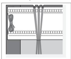
Insert a two-prong curtain hook at the back of each set of pleats. Insert the two prongs into adjacent two pockets and flip the hook on itself as shown.
