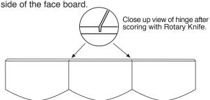
Fold the board along the cut to create a hinge. Ideal for fitting a bay window.
