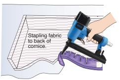
Use 1/2" long staples (Stk.# NS34) or <sup>5</sup>/8" long staples (Stk.# NS35) when stapling into the edge of FirmaFlex™. Shorter staples will not hold as well in the edges.
