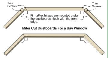
The size of the hinges will depend on the overall size of the window treatment. The hinges should be wide enough to fully support the side boards when the treatment is lifted by the middle board. Recommended size is at least 8" wide x 3" high before scoring. This allows 4" of support under each section of the dustboard.
