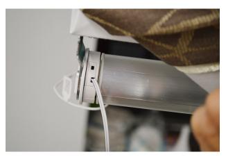
The P1 button on the motor head should face the front of the shade for easy programming
