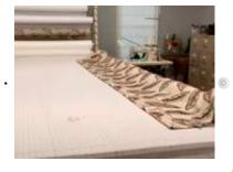
After the panels are folded and banded, they are taken to the appropriate machine to stitch the pleats.
