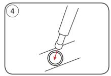
**INSERT POLE TIPS INTO CORNER GROMMETS**
