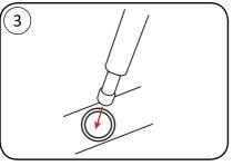
**INSERT POLE TIPS INTO CORNER GROMMETS**
