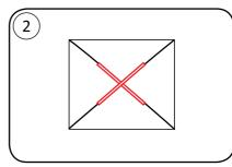
INSERT MAIN POLES THROUGH MIDDLE POLE SLEEVES
