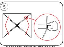
PLACE BROW POLES ON TOP OF MAIN POLES AND INSERT INTO GROMMETS
