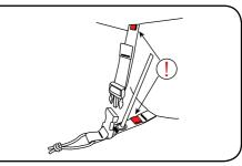
NOTE RED TABS ON FRONT CORNERS CONNECT BUCKLES AND PULL TO TIGHTEN
