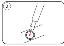
INSERT POLE TIPS INTO CORNER GROMMETS
