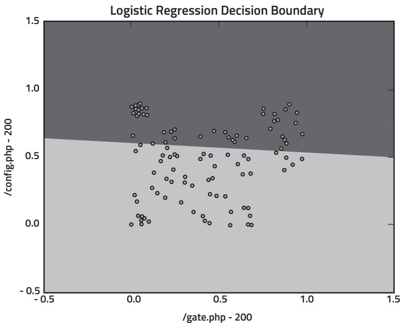
FIGURE 2.1: Decision Boundary in Logistic Regression
