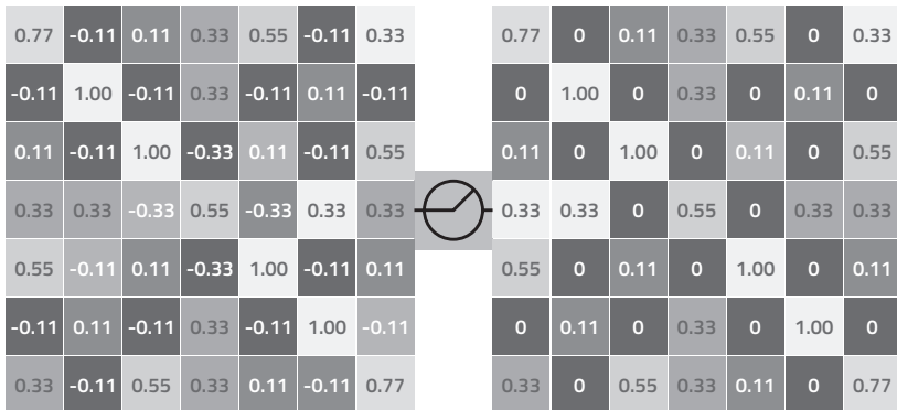
FIGURE 4.13: RELU Layer Converts Negative Values to Zeros
