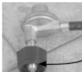
(B) Nipple has to be centered into the LP tank valve
