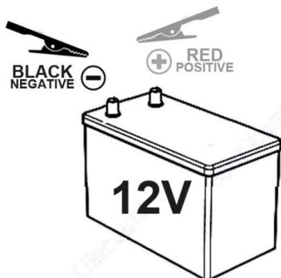
CONNECT THE DIGITAL TIMER TO A 12V RECHARGEABLE BATTERY (NOT INCLUDED) BY ATTACHING THE RED ALLIGATOR CLIP TO THE POSITIVE TERMINAL (+) AND THE BLACK ALLIGATOR CLIP TO THE NEGATIVE (-) TERMINAL.
