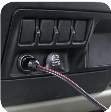
Insert the power adapter into a car's 12V power outlet.
