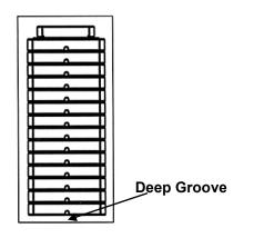
Slide weight plates onto Guide Rod from top to bottom. The deep groove on each weight plate needs to face front and downwards.
