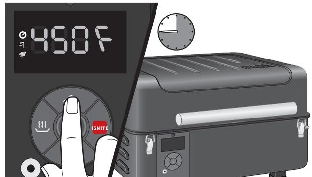
**8** Press the IGNITE button. Let the grill run at 450°F (250°C) for 30 minutes with the lid closed to complete the seasoning process.
