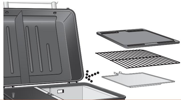
**6** Now you're ready to place the grease drip tray and porcelain-coated grill grates or cast-iron griddle back into the grill. Place the grease bucket under the grease drain on the back of the grill to catch grease drippings.
