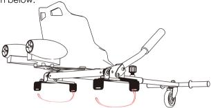
3. Wrap both hook and loop straps under your self-balancing scooter and attach the ends to the hooks on the back of each pedal mount. The rubber protective straps should be centered underneath the hoverboard, with side B facing the ground. One set of rubber protective straps should come pre-assembled with the hook and loop straps.
