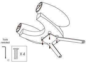
3. Align the holes of the Fog Blaster Mount to the holes of the Frame Base as shown below.
