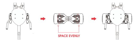
2. Using two Hook and Loop straps, attach one end of each Hook and Loop strap to the holes on the front of each pedal mount as shown below.
