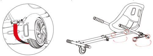
Wrap one set of adjustable straps under your self-balancing scooter and attach the ends of the straps on the back of each pedal mount. The rubber protectors on the straps should be centered underneath the scooter, with side B facing the ground.
