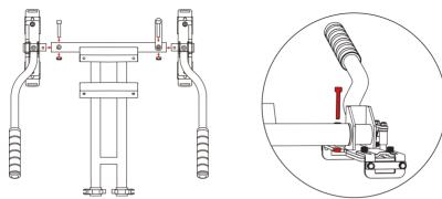
3. Insert the frame into the seat frame. Adjust the foot rest extension and the seat frame to your preferred length. Secure the frame in place using the 2 lockers.
