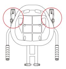
Hoverboard must be calibrated and turned OFF prior to installing buggy.
