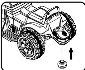
With unit upright, install Bubble Solution Bottle as shown - hand tight.
