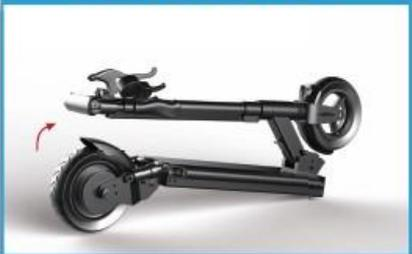
2. Then, unfold the stem of the scooter until the safety bar clips into place. Give the stem an extra push to ensure the safety bar is locked into place.
