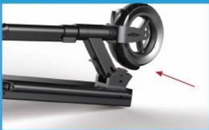
1. First lift up the latch, releasing the safety bar.
