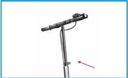
3. Finally, unscrew the handlebar folders, open them up and screw them back into place. Also ensure the latch on the stem is tightened after adjusting it to the correct height.
