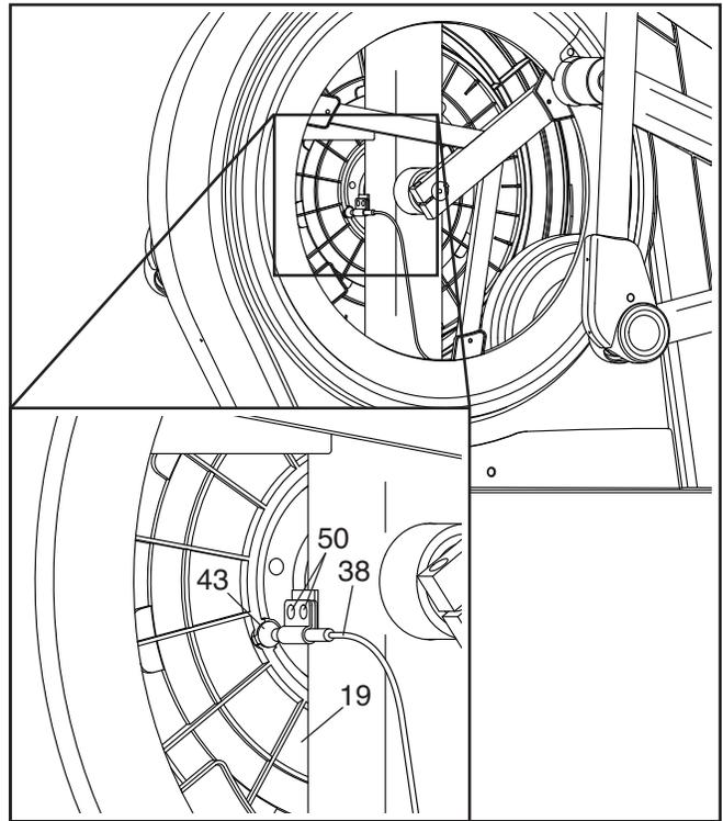
Next, slightly loosen the two indicated M4 x 13mm Self-tapping Screws (50). Slide the Reed Switch (38) slightly closer to or away from the Magnet (43), and then retighten the Screws.
