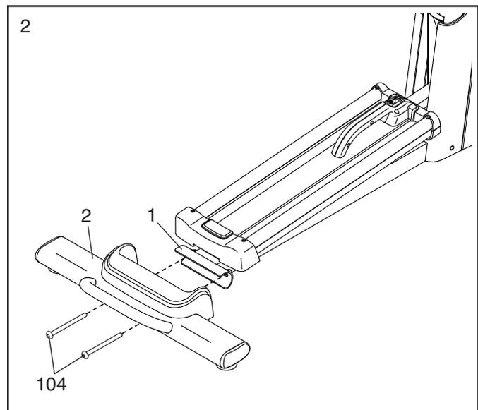
3. With the help of a second person, place some of the packing materials (not shown) under the front of the Frame (1). **Have the second person hold the Frame to prevent it from tipping while you complete this step.**
