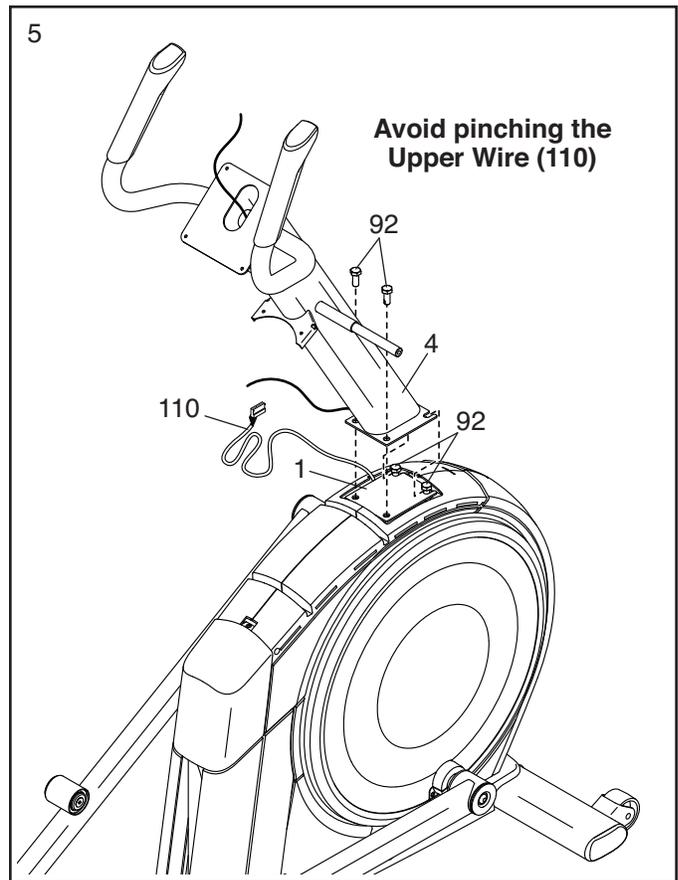
6. Locate the wire tie (A) in the lower end of the Upright (4). Tie the wire tie to the Upper Wire (110). Then, pull the upper end of the wire tie until the Upper Wire is routed through the Upright.
