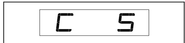
**Demo Mode**—The currently selected demo mode option will appear in the display. The console features a demo mode, designed to be used if the elliptical is displayed in a store. If the demo mode is turned on, the console will not turn off and the display will not be reset when you finish exercising. Press the Resistance increase button repeatedly to select a demo mode option. To turn on the demo mode, select DON. To turn off the demo mode, select DOFF.
